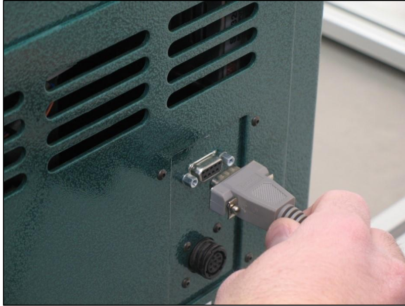
Figure 22: Inserting a 9-Pin “D” End of the PN 9580 External 9-Pin “D” Cable into the PN 9583 Coiler Accessory Board Kit
