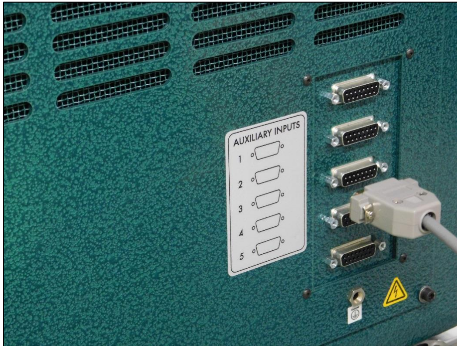
Figure 31: Inserting the 15-Pin “D” Foot Switch Assembly Connector into the PN 9686 Accessory Board Kit
