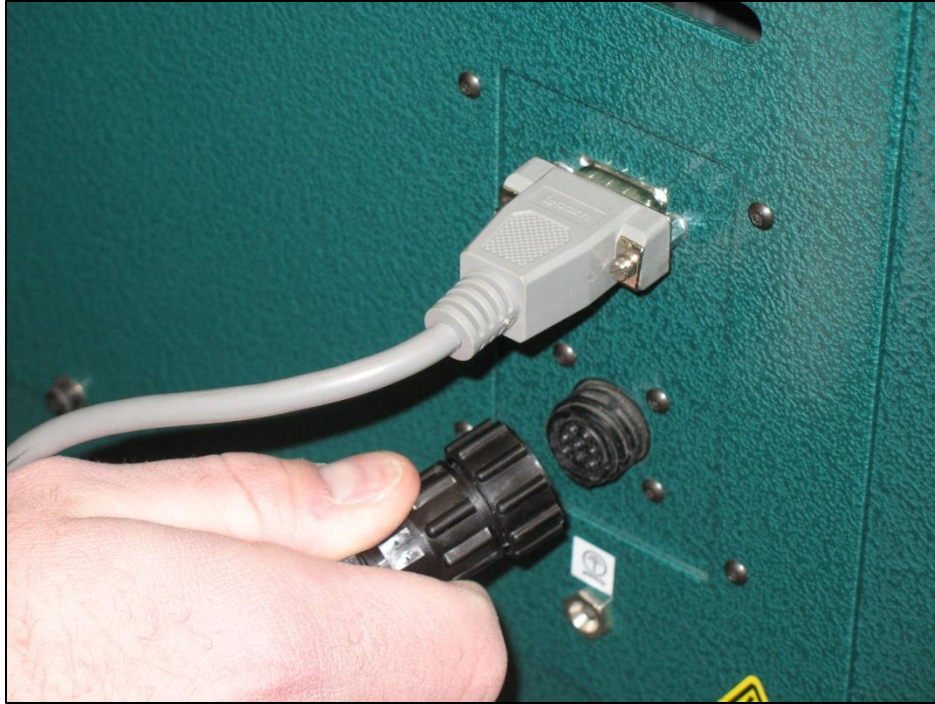
Figure 32: Inserting the Foot Switch Assembly Connector into the PN 9583 Coiler Accessory Board Kit
