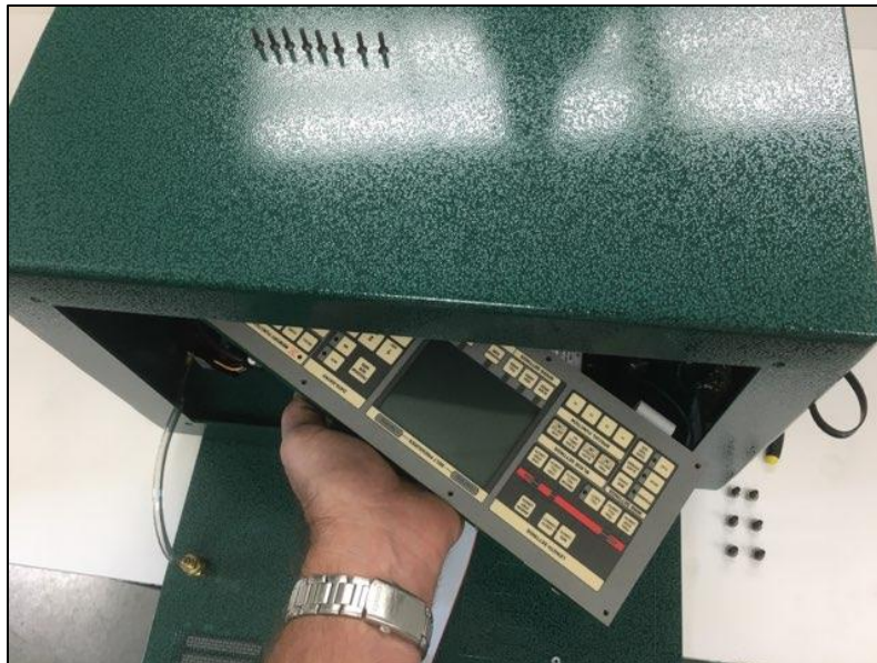
Figure 8: Reinstalling the Front Panel
