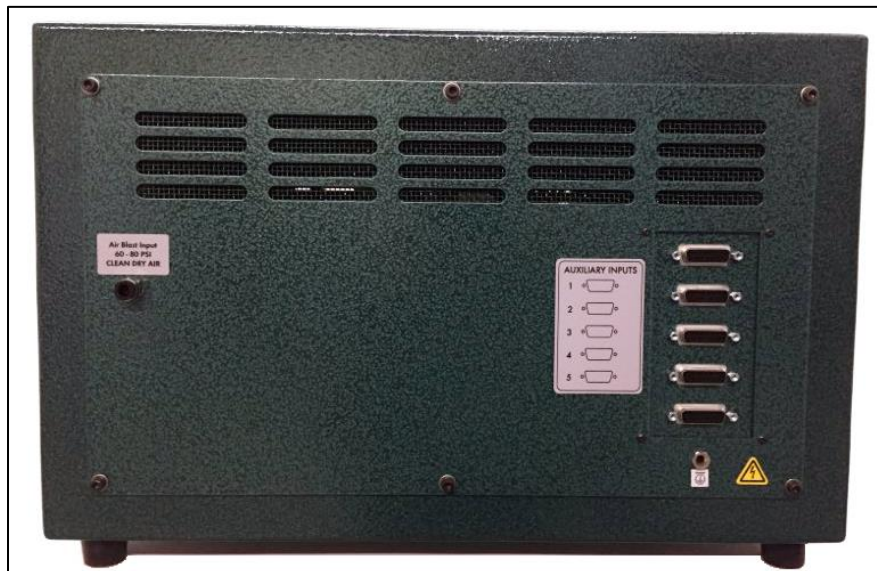
Figure 11: PN 9686 Accessory Board Kit Assembled
