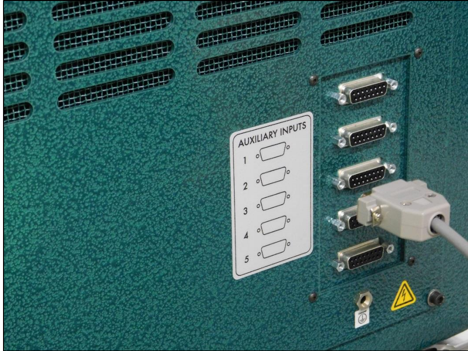
Figure 21: Inserting the 15-Pin “D” End of the PN 9614 Coiler Interface Cable into the PN 9686 Accessory Board Kit
