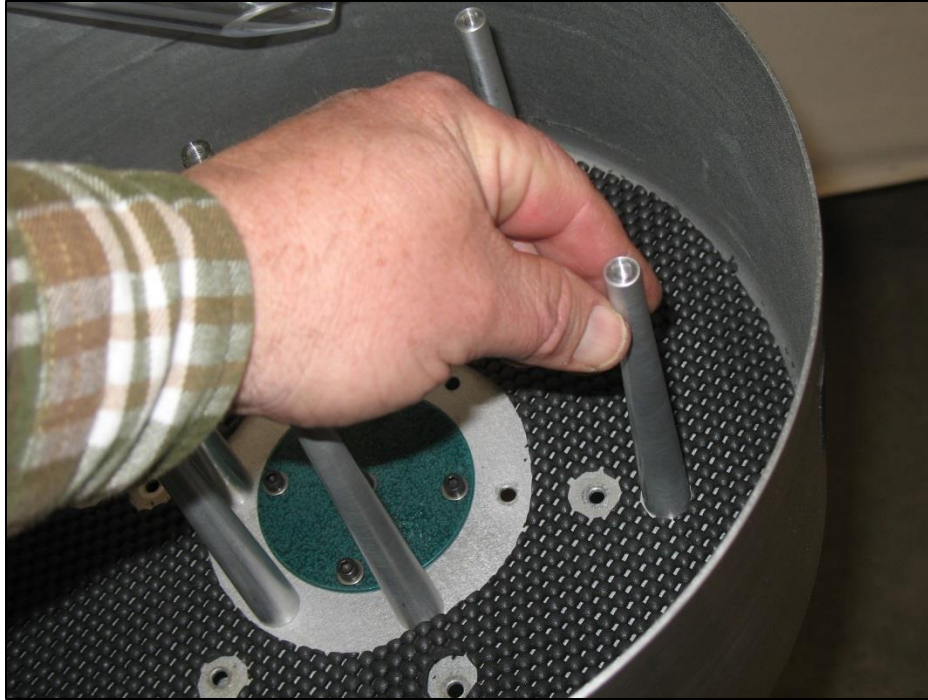
Figure 35: Repositioning the (6) PN 9517 Ring Stand-Offs
