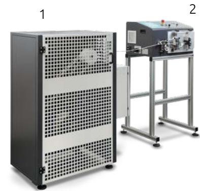
Inline assembly example: 1 Motorized dereeler 2 Cut, strip & unjacket machine
